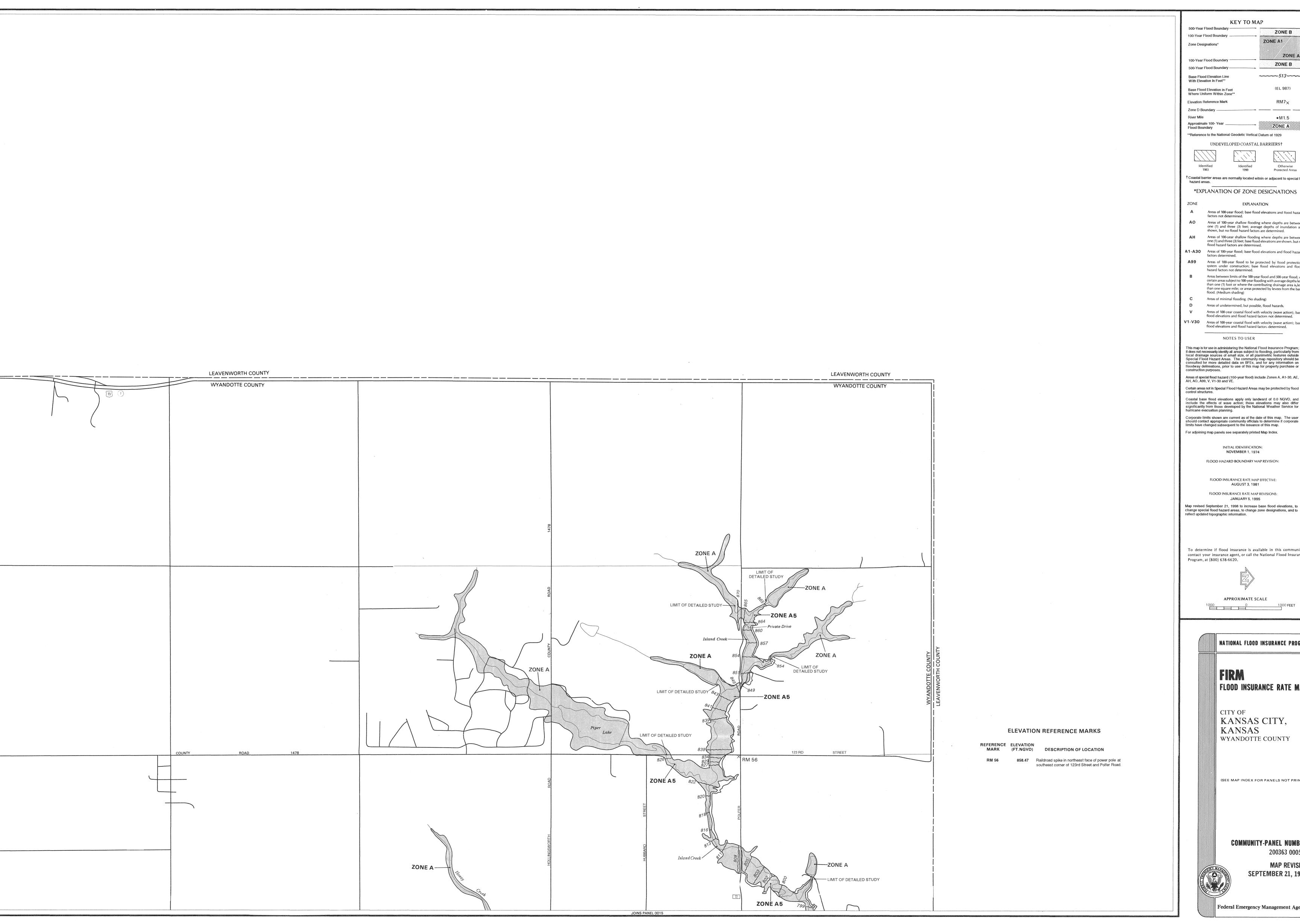
KEY TO MAP 500-Year Flood Boundary ----ZONE B 100-Year Flood Boundary -ZONE A1 Zone Designations\* ZONE A5 100-Year Flood Boundary — ZONE B 500-Year Flood Boundary — ----513----Base Flood Elevation Line With Elevation In Feet\*\* (EL 987) Base Flood Elevation in Feet Where Uniform Within Zone\*\* Elevation Reference Mark  $RM7_{\times}$ Zone D Boundary ----River Mile ●M1.5 Approximate 100- Year \_\_\_\_\_ ZÔNE A Flood Boundary \*\*Reference to the National Geodetic Vertical Datum of 1929
